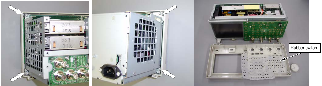
Figure 6-6: Front case removal
