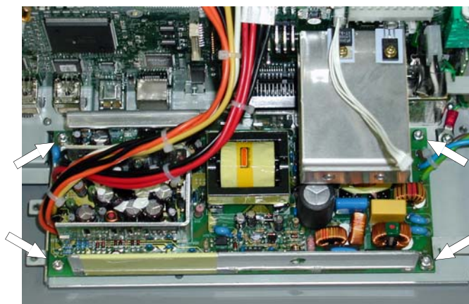
Figure 6-15: Power supply removal
