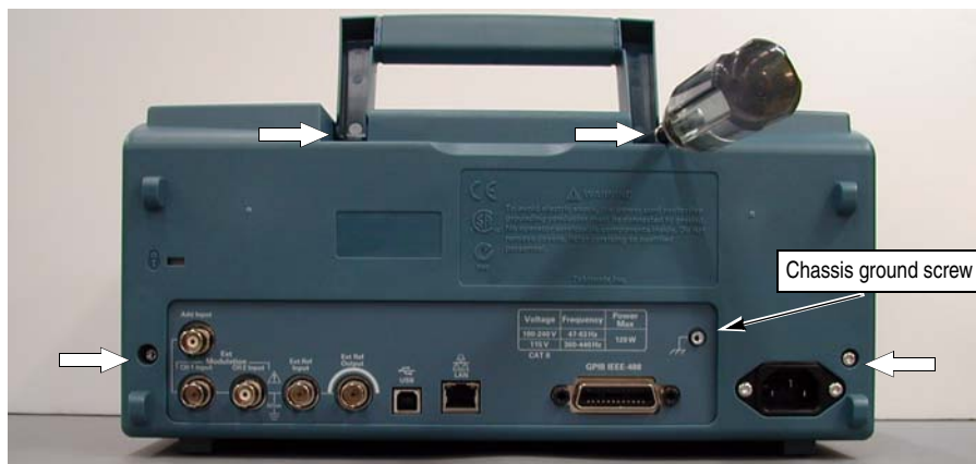
Figure 6-3: Rear case removal
