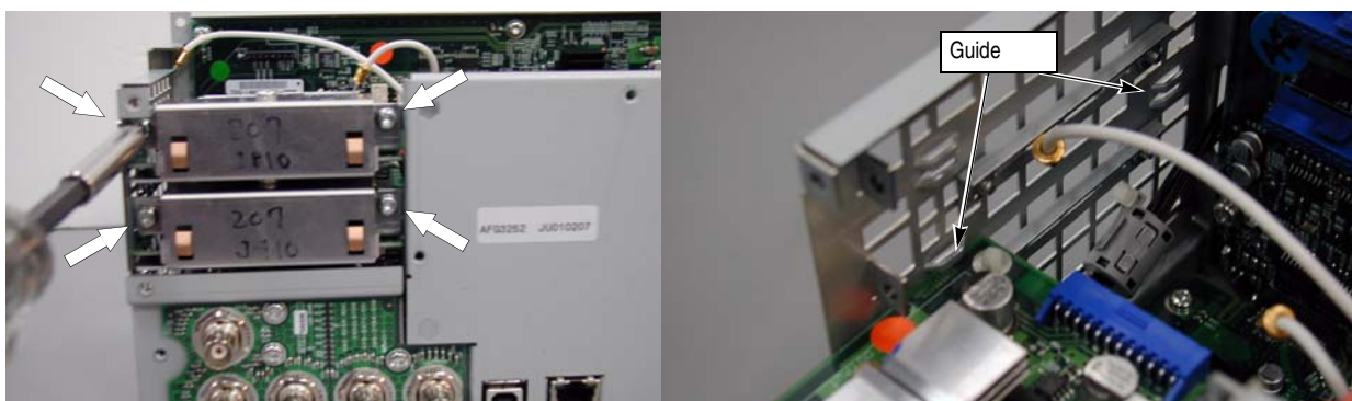
Figure 6-9: Output board removal
