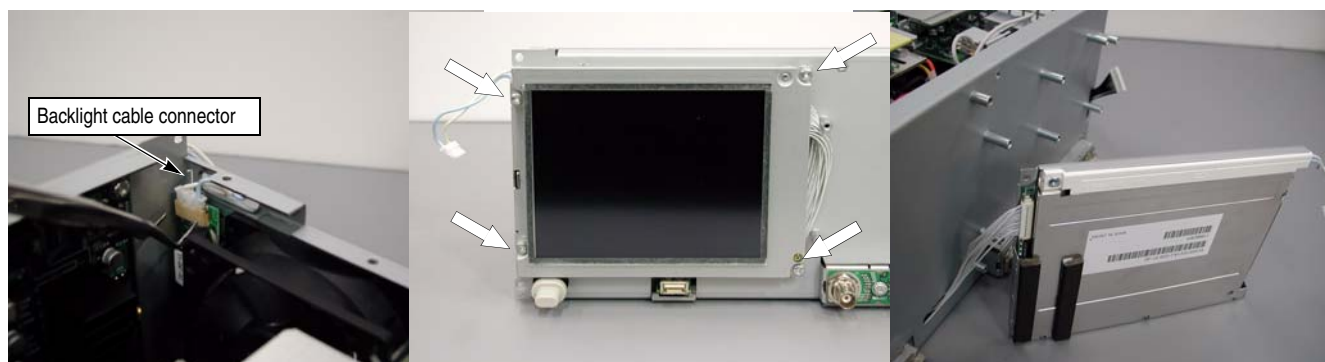
Figure 6-8: Display module removal
